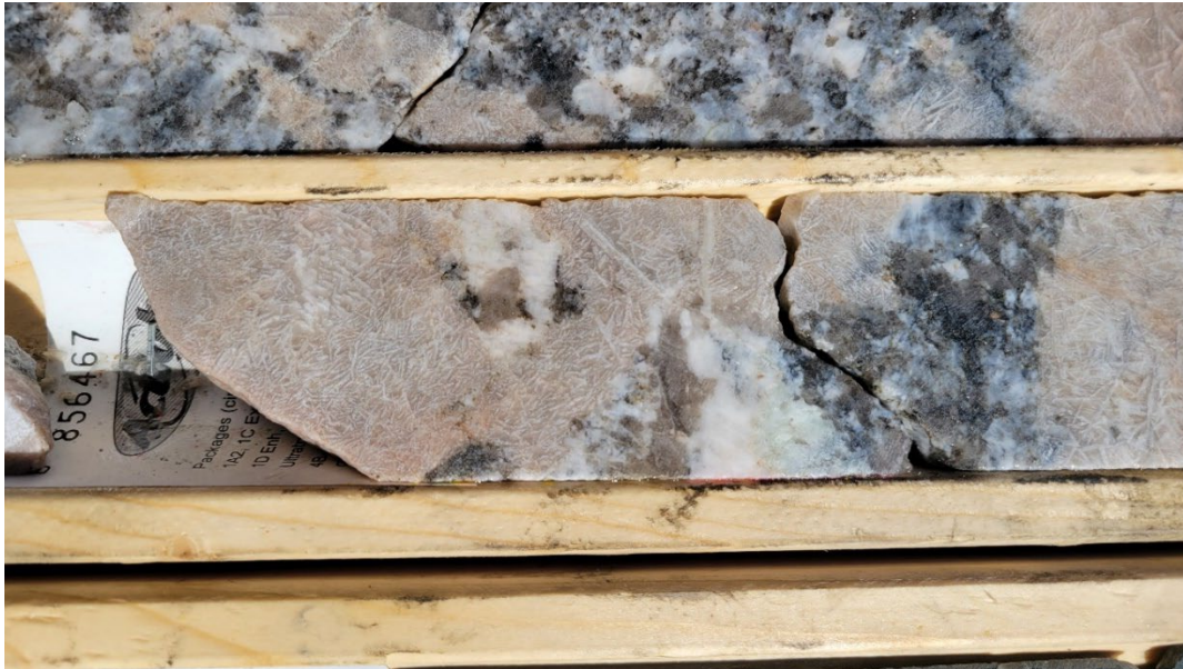
Above: Close up of lithium-bearing spodumene quartz intergrowth (SQUI) in GLD22-02. The one metre sample assayed 2.28% Li 2 O.
