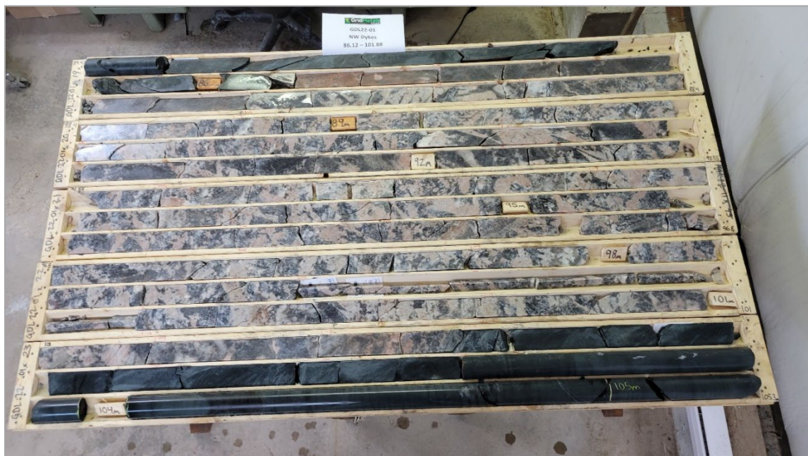
Above: Northwest dyke intersection in drill hole GDL22-01, Donner Lake property. NQ core size.
