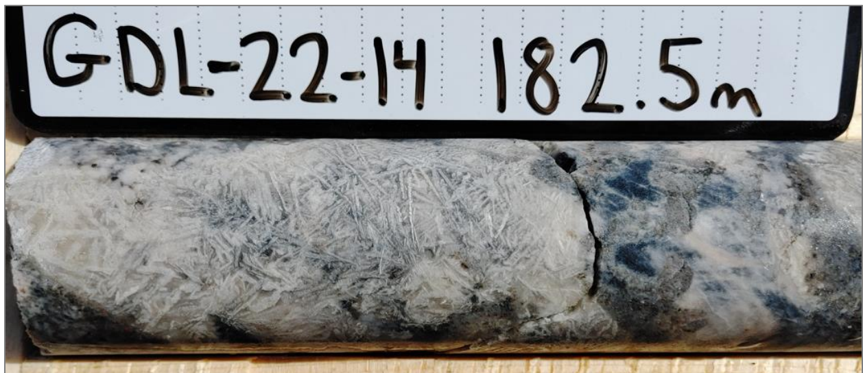
Above: Spodumene-quartz intergrowths (SQUI) from GDL-22-14 at 182.5 meters downhole.
