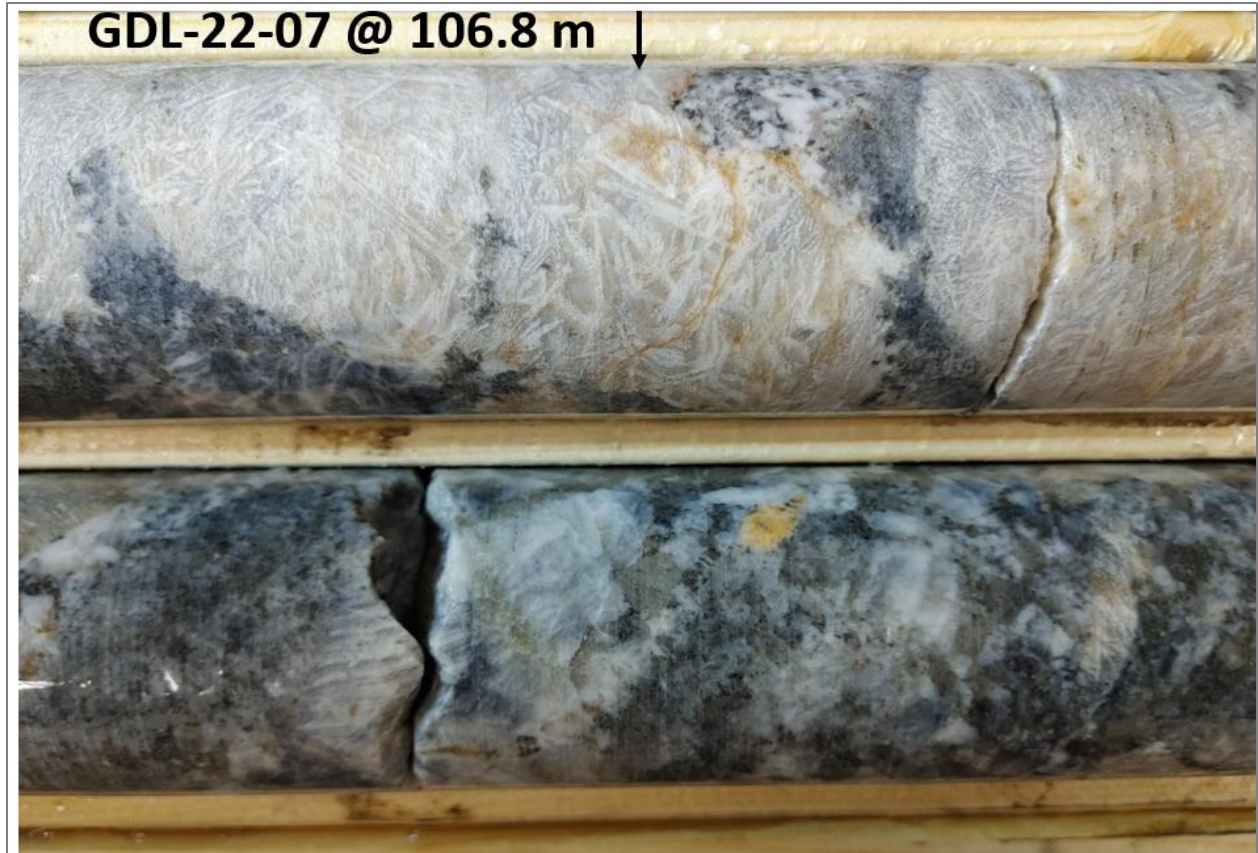
Above: White spodumene blades in GDL-22-07 at 106.6 meters downhole.
